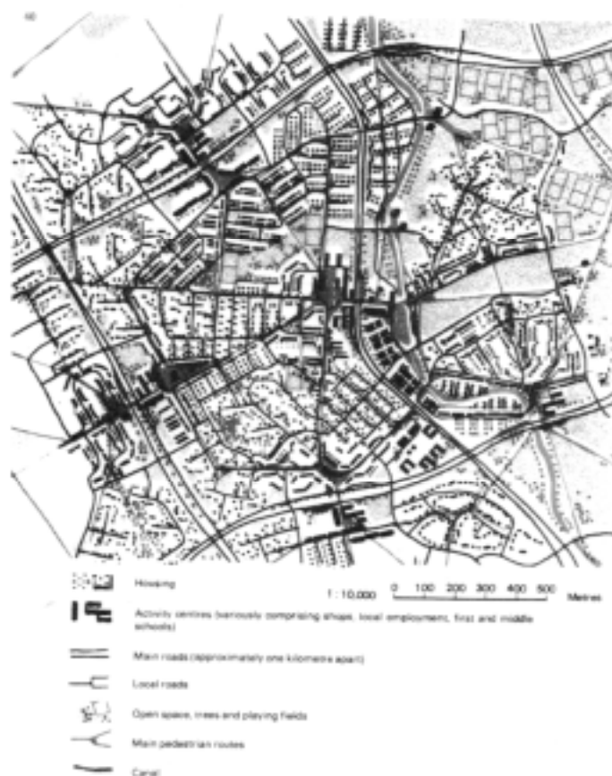
Figure 7. An impression of a part of the city. The proposals for planning the local environment are illustrated on this sketch which shows how a typical part of the city might be developed
