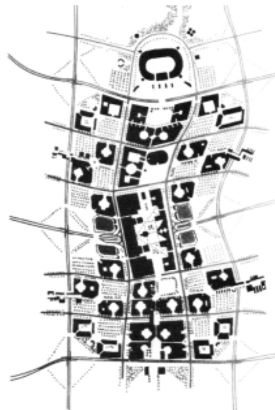
Figure 8. The environment of the new city centre. A possible layout is shown for roads, buildings, main pedestrian routes and main planted areas. In the centre is a climate-controlled shopping mall linked to public buildings, offices and housing
